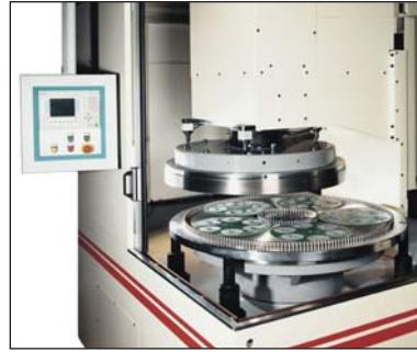
Flathoning machines are unlike conventional fixed abrasive grinders used for sizing components. Clean lapping far exceeds the 0.0002-in to 0.0003-in tolerances of conventional grinders. A smaller machine can finish up to 100-150 inserts within 7-8 minutes, a rate of 700-1000 parts per hour.
