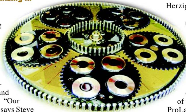
Using the Stahli DLM700, ProLap is able to produce parts with tolerances of  $\pm 0.00008"$  ( $\pm 2\mu$ ) and 2 – 4 Ra surface finishes.
