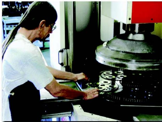
The Stahli DLM700 is a double-sided flat-honing machine featuring a unique dual wheel design enabling both sides of flat pieces to be ground simultaneously with fixed abrasives.
